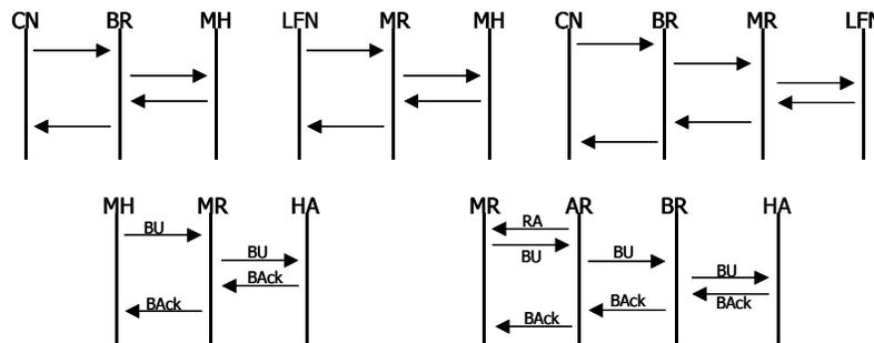
**Figure 13: Initial Exchanges and Tunnel Setup, Mobile Network and Mobile Host**
