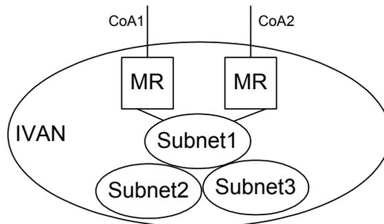
**Figure 38: Multi-homed moving network with multiple mobile routers, several IP subnets**
