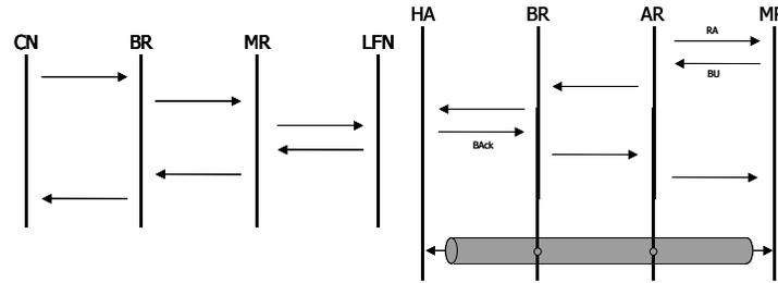
**Figure 10: Initial Communication and Tunnel Setup for Simple Mobile Networks**
