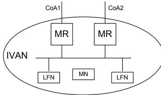
**Figure 37: Multi-homed moving network with multiple mobile routers, one IP subnet**
