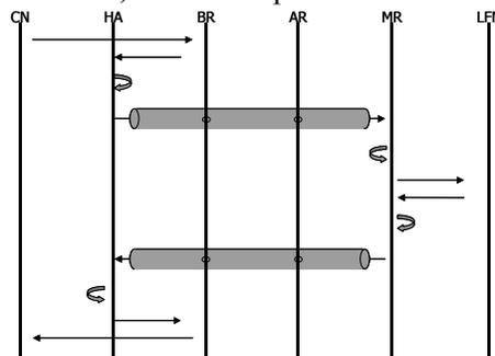
**Figure 11: CN-LFN Exchanges, Simple Mobile Networks**
