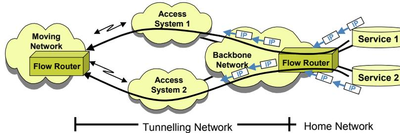
**Figure 33: Flow routing for multi-access mobile networks**
