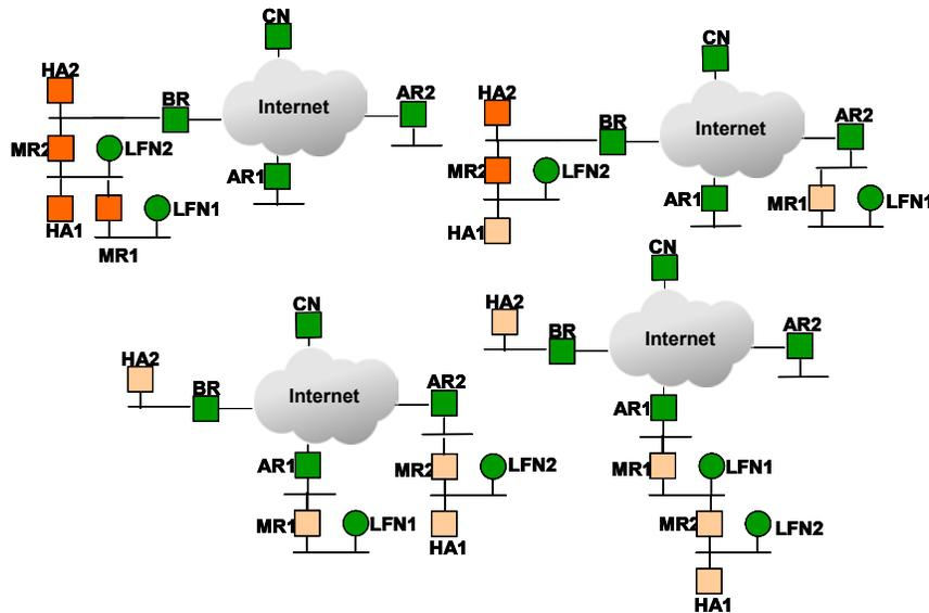
**Figure 31: Nested Mobile Networks with “Crossover” Tunnels**
