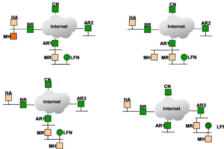
**Figure 21: Mobile Network and Mobile Host at Same Home, Both Move, Initially Separated**
