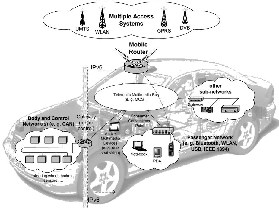
Figure 1: In-vehicle communication architecture
