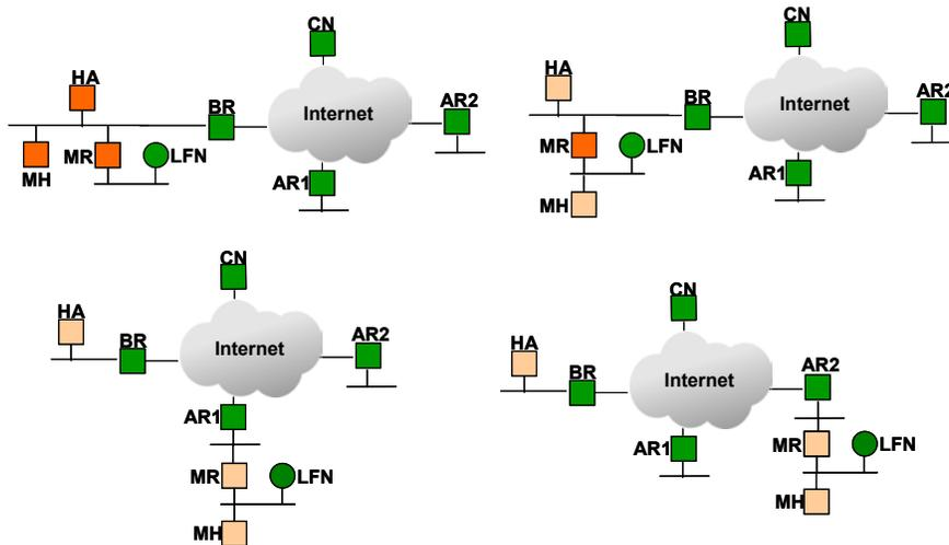
**Figure 19: Mobile Network and Mobile Host at Same Home, Both Move, Homogeneous**
