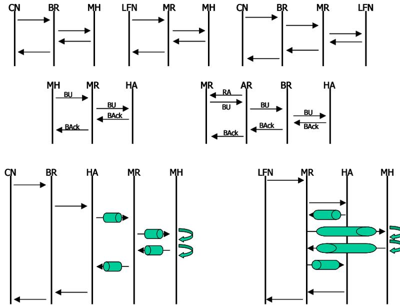
**Figure 20: Initial Communication, Tunnel Setup, Subsequent Communication**
