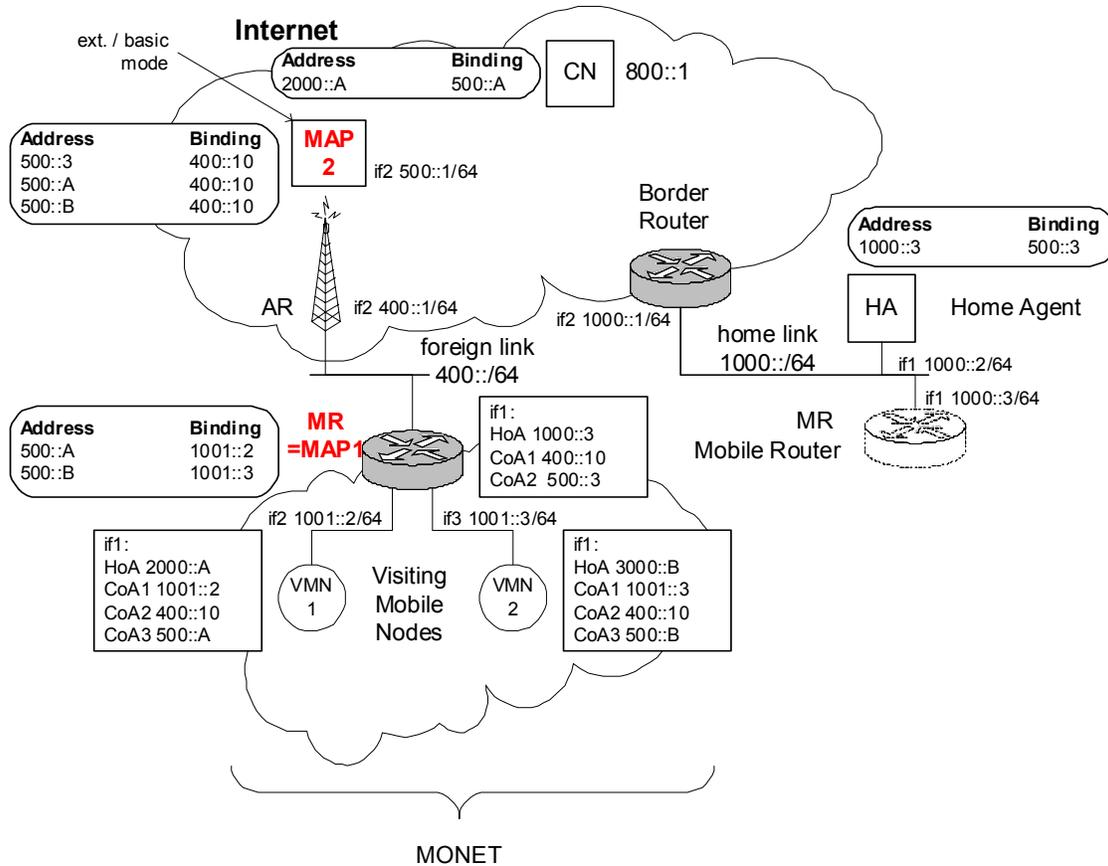
**Figure 9: Mobile networks with HMIPv6**
