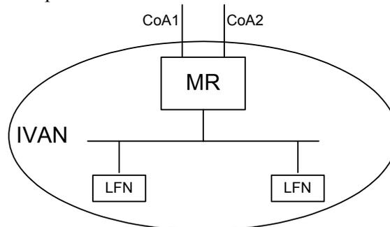
**Figure 36: Multi-homed moving network with one mobile router**
