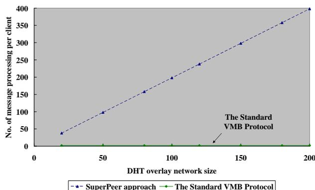
Figure 90 – No. of message processing per node Vs. DHT overlay network size
