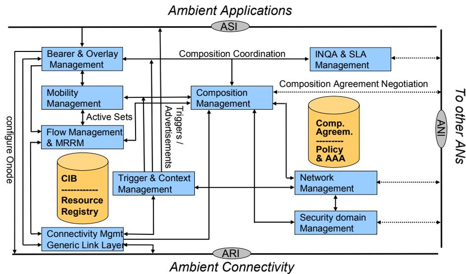
Figure 49 – Interaction diagram for Multi-Radio Resource Management (MRRM)
