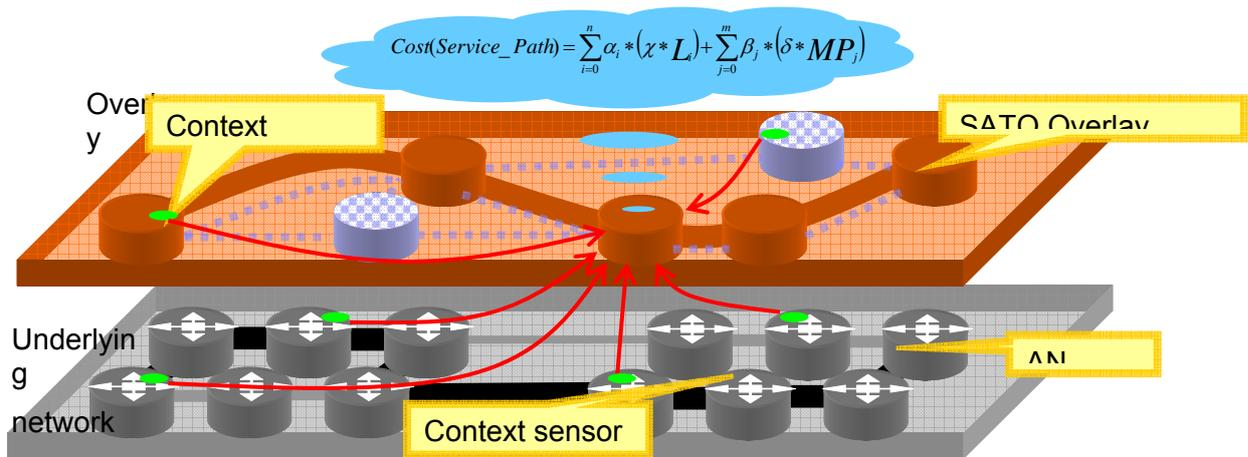
Figure 30 – Use of context sensors in overlay routing
