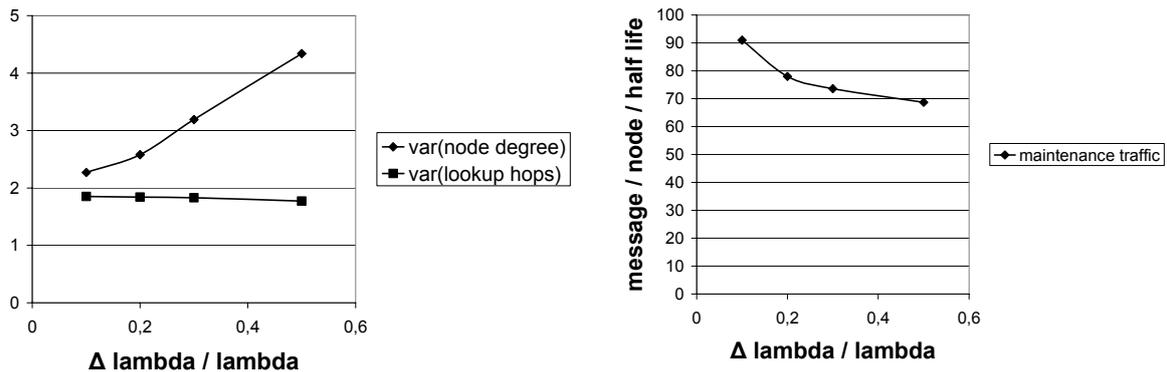
Figure 88 - Effect of  $\Delta\lambda$  on maintenance overhead and variance of node degree and lookup hop count
