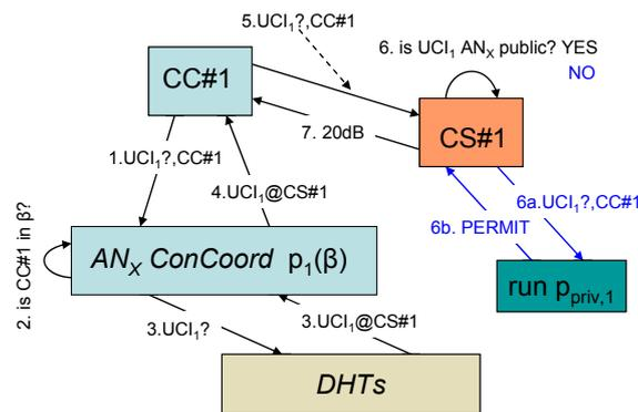
Figure 66 – ContextWare access control within a single AN (security domain)
