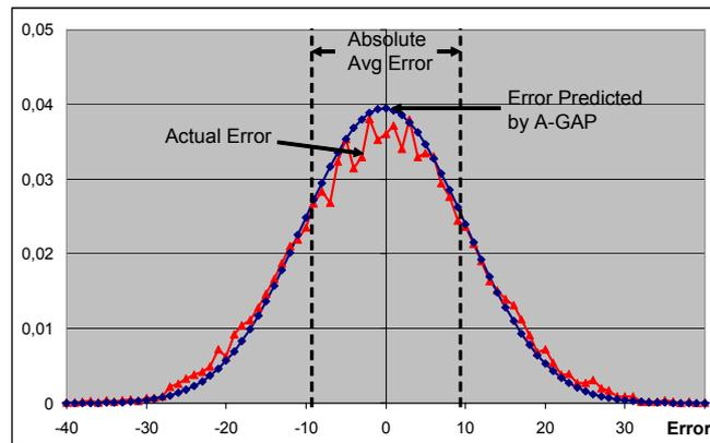
Figure 33 – Distribution of the error predicted by A-GAP and the actual error at the root node
