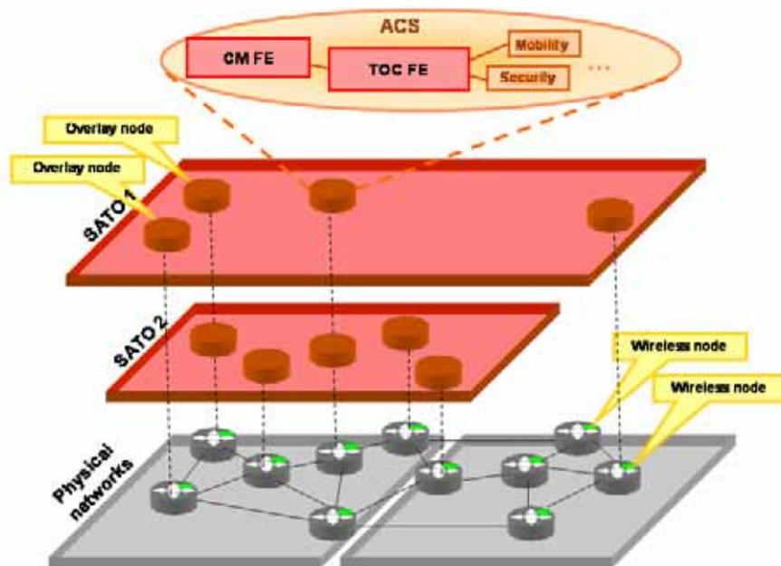
Figure 50 – An illustration of the ACS with example establishments of SATOs
