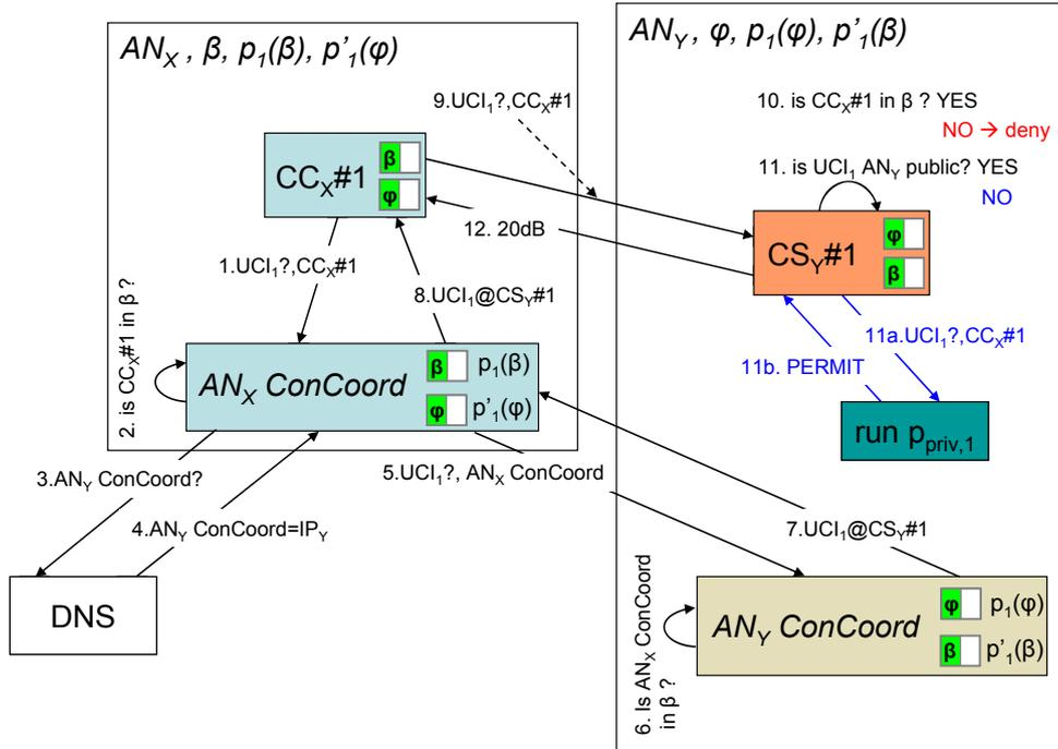
Figure 67 – Inter-AN ContextWare communication and access control
