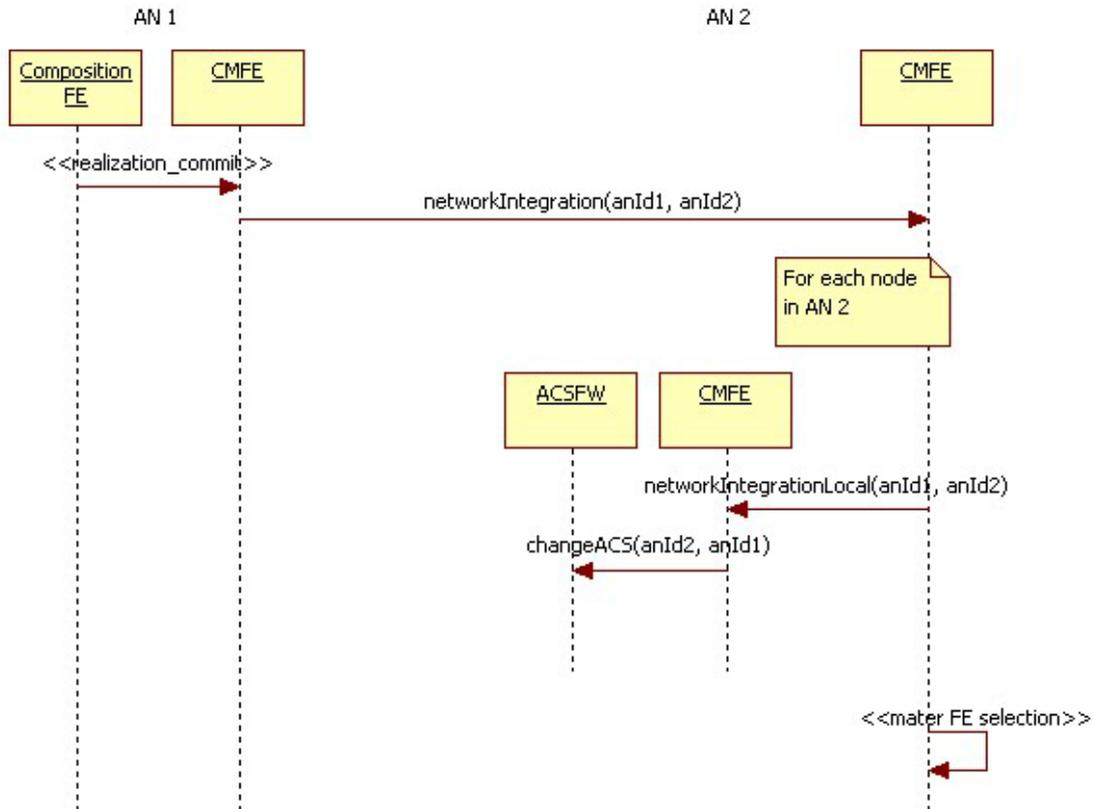
Figure 40 – Interactions of Composition Management FE with other FEs in case of network integration
