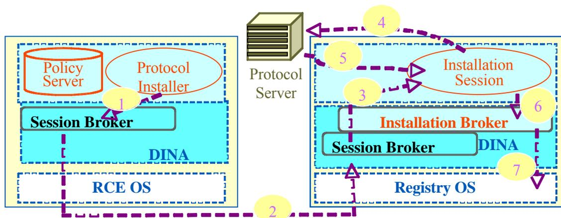
Figure 26 – Protocol Deployment using DINA
