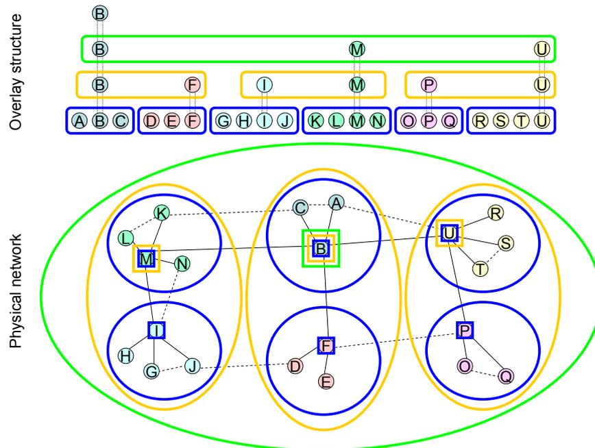
Figure 73 – Overlay and physical structure example – in this case using the echo on the overlay structure would lead to fewer messages in the physical network
