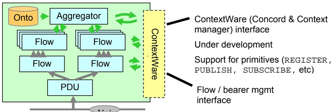
Figure 27 – Basic architecture of flow context sensor
