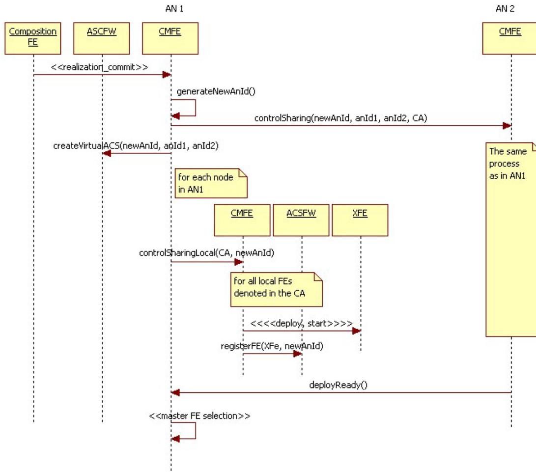
Figure 39 – Interactions of Composition Management FE with other FEs in case of control sharing
