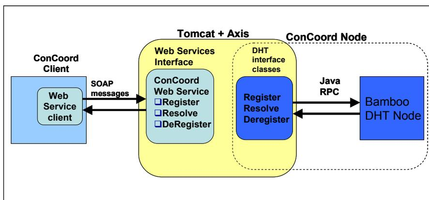
Figure 17 – Illustration of the interactions between a ConCoord client and the ConCoord using the Web Services interface
