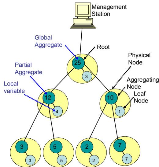
Figure 31 – Example of an aggregation tree with aggregation function SUM
