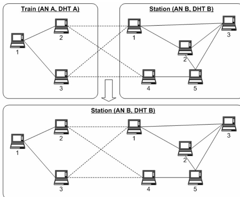
Figure 74 – Composition through absorption
