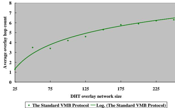
Figure 91 – Average overlay hop count Vs DHT overlay network size
