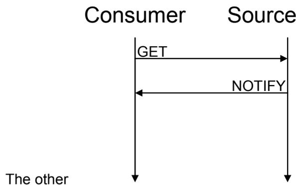
Figure 11 is used when a consumer wants to retrieve the context information when the information is updated. Figure 12 shows the case of a subscribe message being sent to the source and the source replying with notify messages whenever the context information changes. This solution will minimize the traffic as the requesting node will not have to periodically poll the source for updates, instead the source will notify the subscribing consumer when context information is updated.
