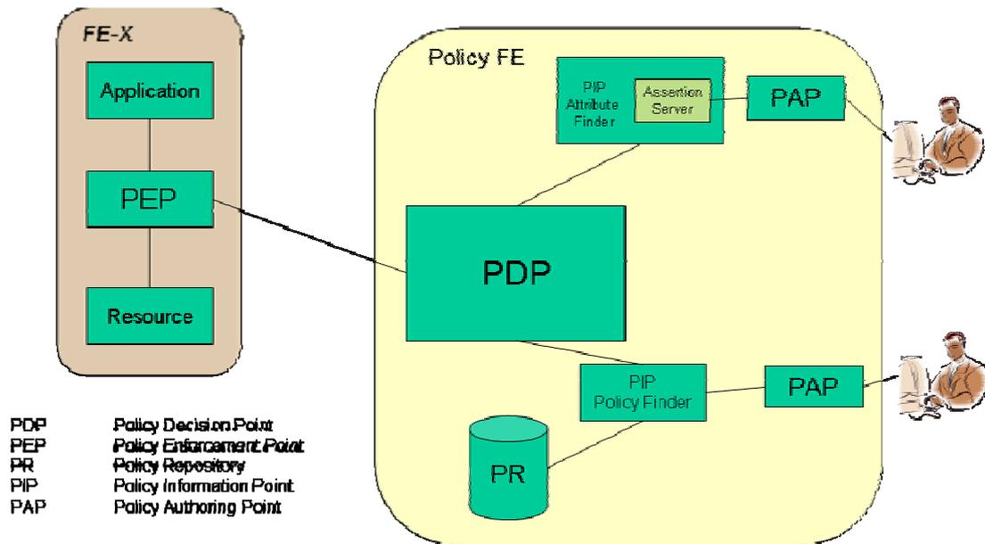
Figure 41 – Components of the basic AN Policy Framework
