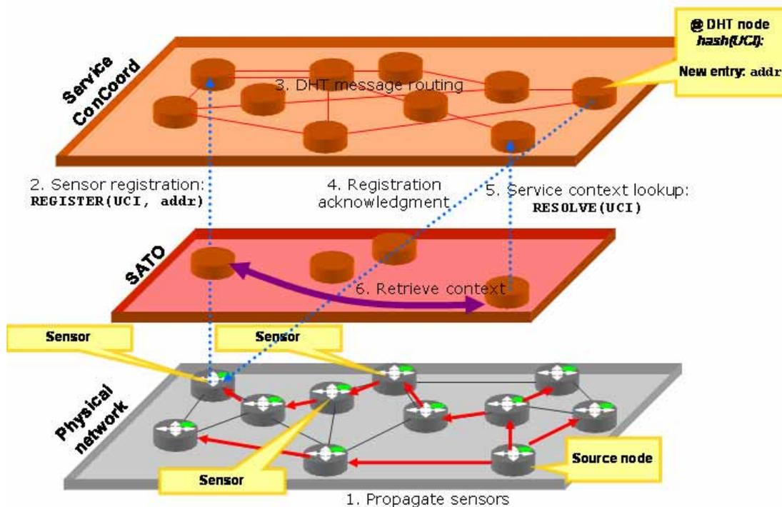
Figure 56 – An illustration of the inter-working between SATO LM and ConCoord
