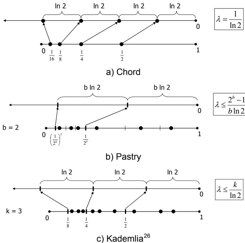
Figure 89 – Derive long-range connection density of various DHTs by inverse transformation
