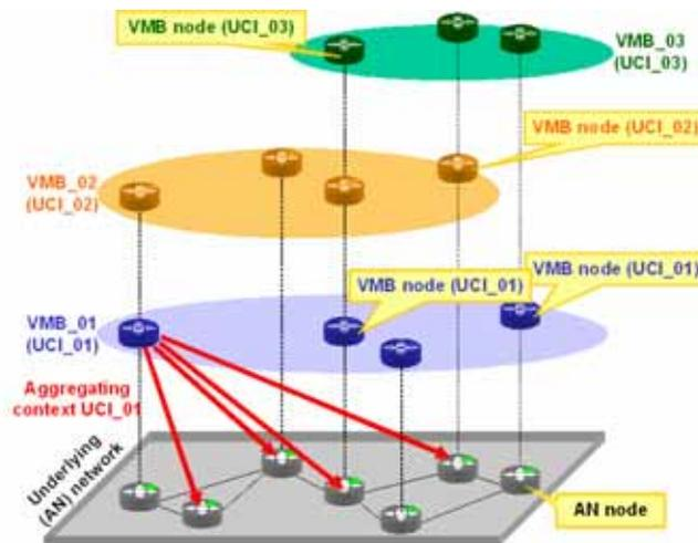
Figure 57 – Different VMB nodes and VMBs in an AN
