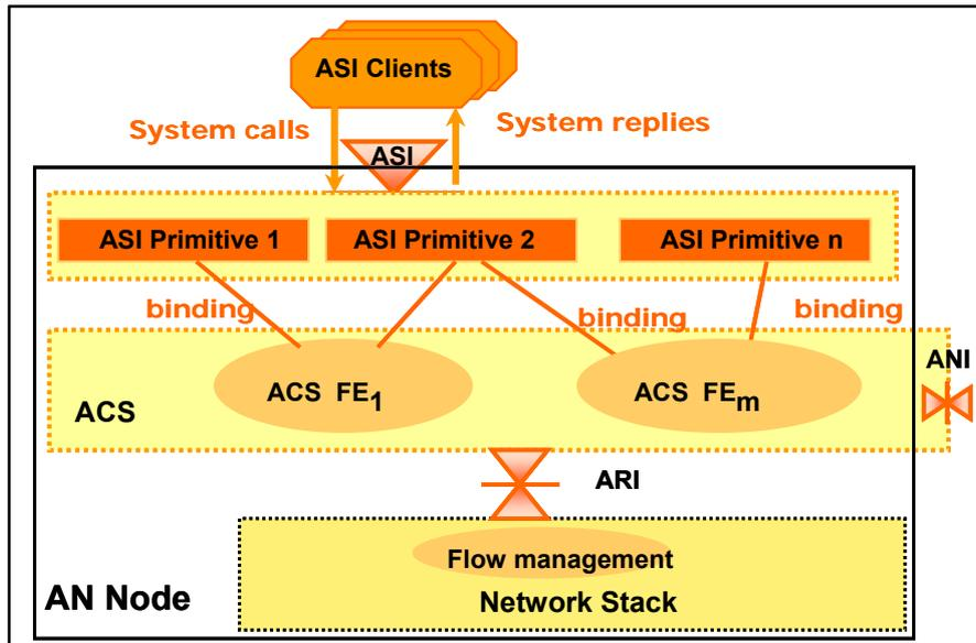
Figure 53 – Diagram depicting the bindings between the Functional Entities and the ASI primitives
