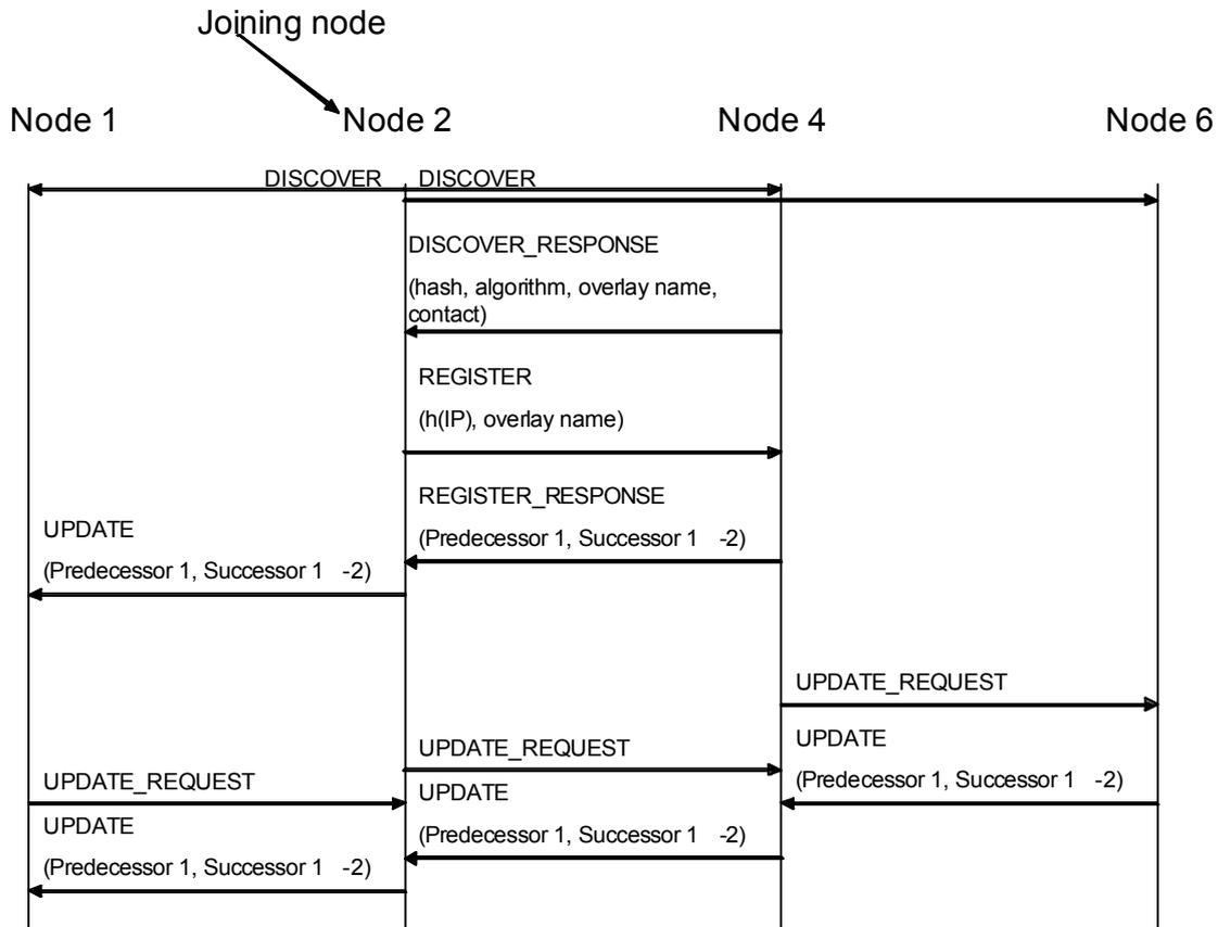
Figure 6 – A CUA registering in a DHT overlay
