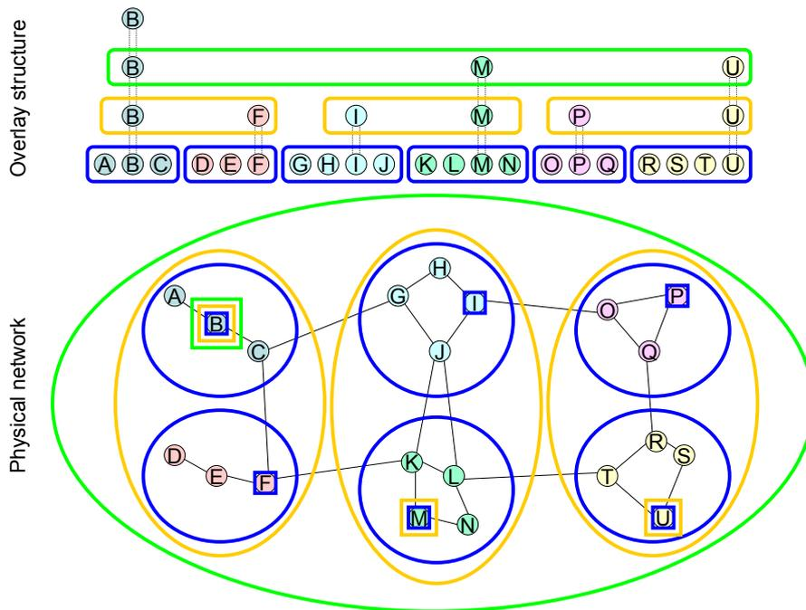
Figure 72 – Overlay and physical structure example – in this case using the echo on the physical structure would lead to fewer messages in the physical network
