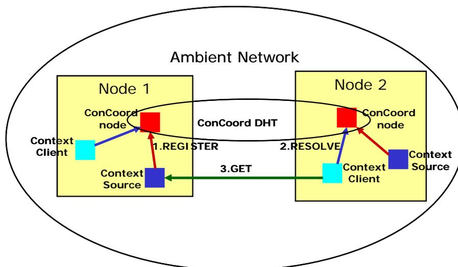
Figure 16 – Illustration of the interactions between context clients, sources and the ConCoord in an Ambient Network
