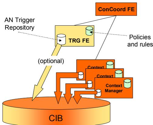
Figure 48 – Diagram showing the integration of ContextWare and the Triggering FE
