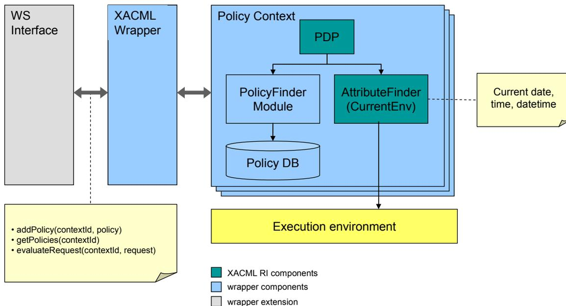
Figure 43 – Architecture of the XACML Wrapper
