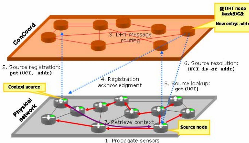
Figure 52 – An illustration of the inter-working between SATO LM and ConCoord
