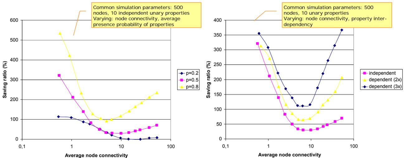
Figure 71 - Evaluation of property set based self-organization algorithm for unary properties
